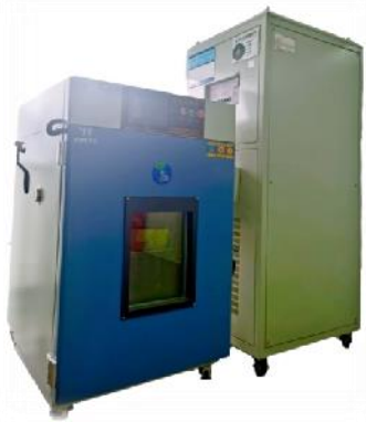
Ripple current test power supply
