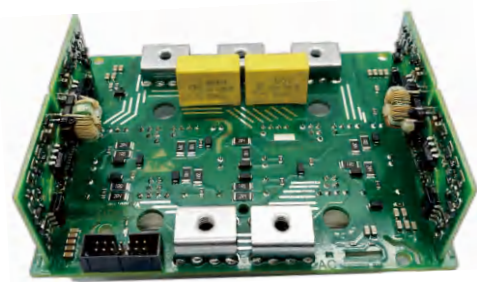
Two IGBTs in parallel installation unevenness <50um
